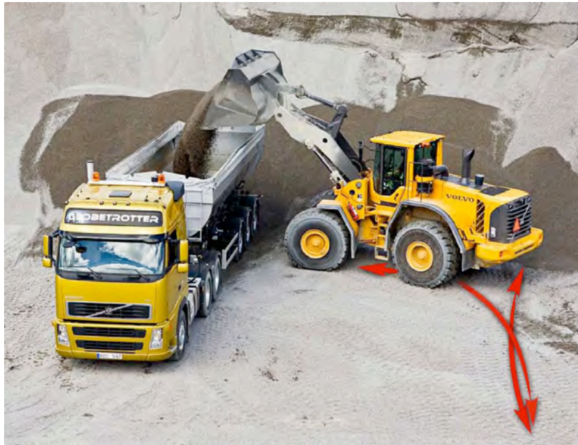
Figure 3: Short loading or Y-cycle of a wheel loader
